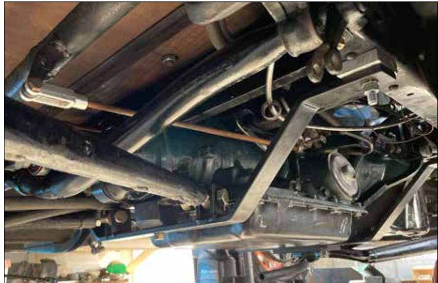
We fabricated a steel strap to support the radius rods and another to support the wishbone up front.
