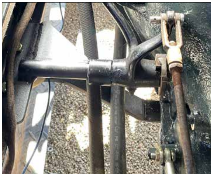
We had to account for the new clearance for the relocated brake pedal.
