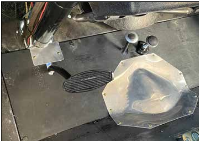
Modifications included shaping a plate to follow the curve of the transmission and align with the floorboards.
