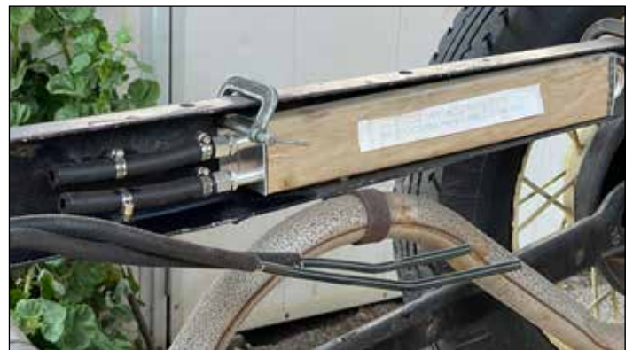
Transmission radiator nestled in frame siderail.
