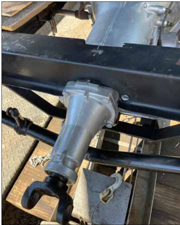
Accommodating the length of the transmission body required removing a portion of the leading edge of the frame's cross member.
