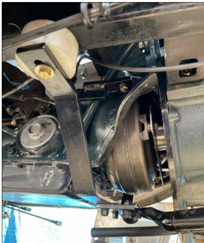
Tight clearance to the wishbone required transmission cover modification.
