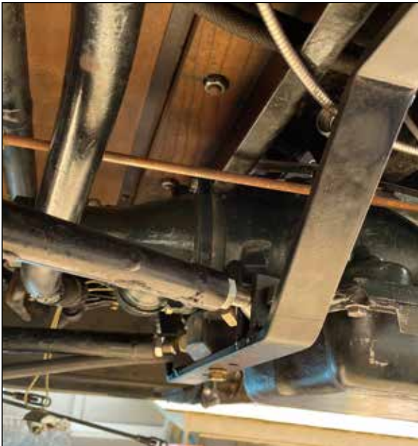
We fabricated a steel strap to support the radius rods and another to support the wishbone up front.
