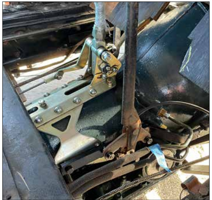
One beauty of the Lokar shifting assembly is how the mounting bracket attaches to the top of the transmission.
