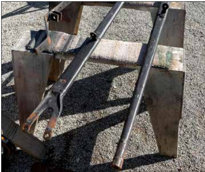
We reinforced the rear radius rods, welding steel rods to their interior.
