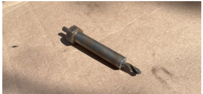
Model T Headbolt drilled for 3/16" bit.
